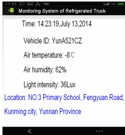
Fig. (8). Environment information inside a transport vehicle from a gateway android smartphone.
