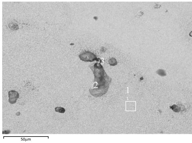
Fig. (2). Microstructures of hardened Fe-Al-Mn grinding ball.
