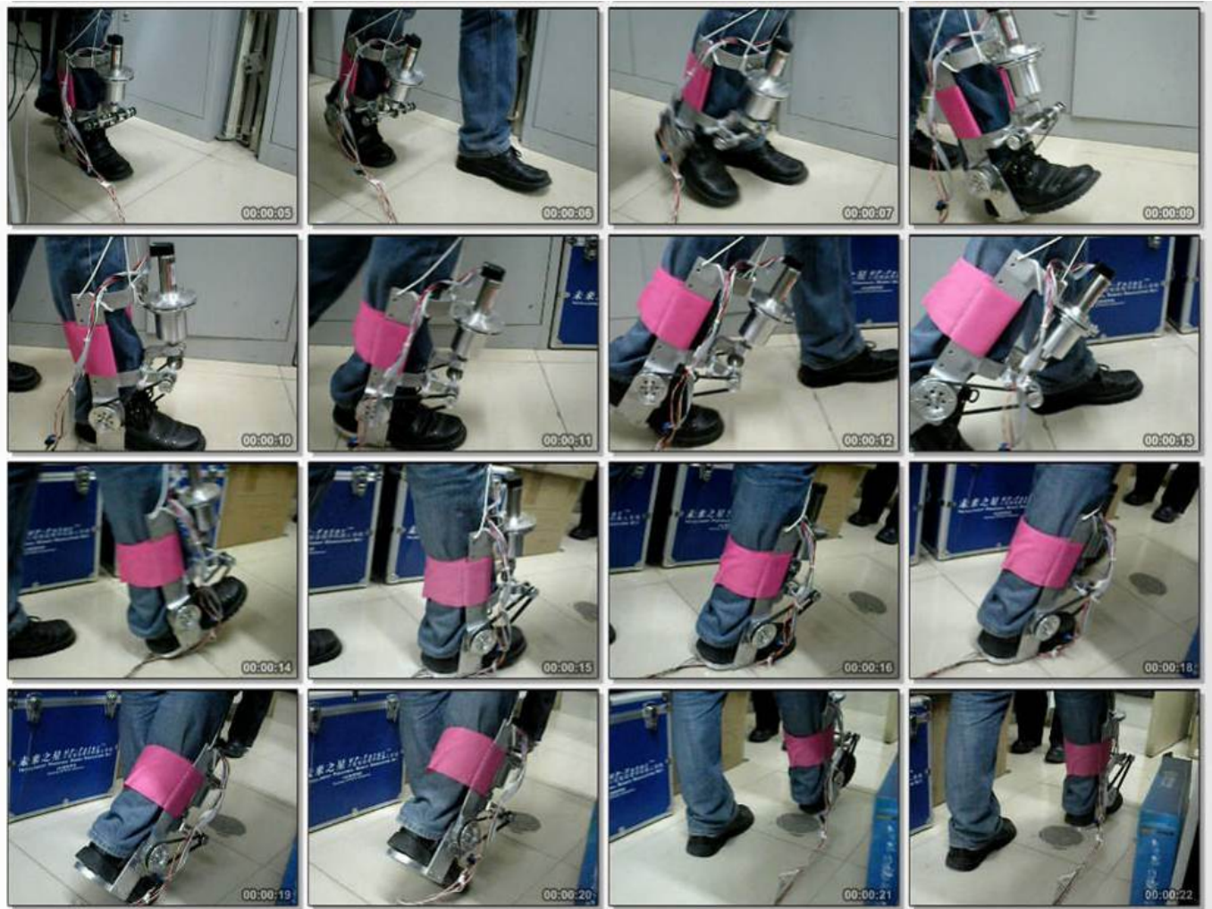
Fig. (13). Motion experiment in walking-aid mode.
