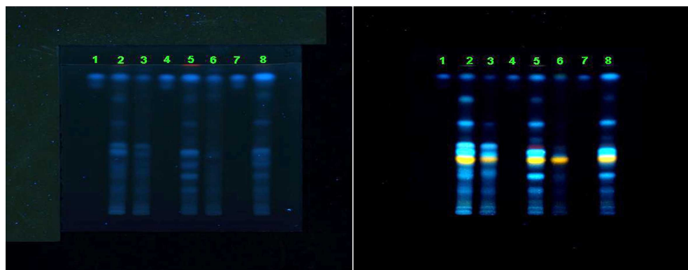
Fig. (3). HPTLC Profiles of Aqueous Extracts of Search-Me-Heart and Marker Compound (Caffeic Acid). 1, 4, 7 - Caffeic Acid (Marker), 2 - SMH/71/2, 3 - SMH/71/76, 5 - SMH/71/116, 6 - SMH/71/147, 8 - SMH/82/28. SMH/71/2 - Location 1, SMH/71/76 - Location 2, SMH/71/116 - Location 3, SMH/71/147 - Location 4, SMH/82/28 - Location 5.
