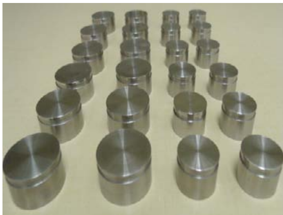
Fig. (1). DIFF-bolts two sizes were trialed 2.54 cm and 1.91 cm. The SFASU DIFF-bolt development team included: Lucinda Choules, Dr. Dennis A. Gravatt, Clay Watts and Ron Havner.
