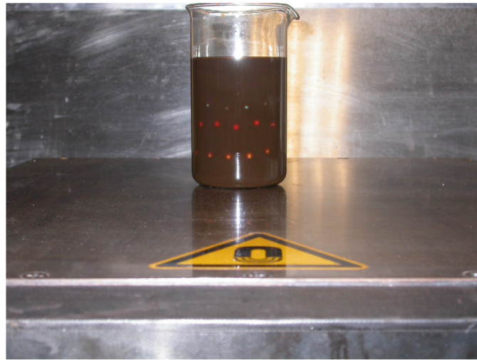
Fig. (3). Picture of plastic particles floating in a magnetic liquid. The liquid is placed in the magnetic field of the magnet which is perpendicular to the surface. This results in different apparent densities at different distances from the surface of the magnet. In this way the particles with the lowest density are floating at the highest position (blue particles). The particles with the highest density are the closest to the surface of the magnet (yellow particles), while the red particles are in between.
